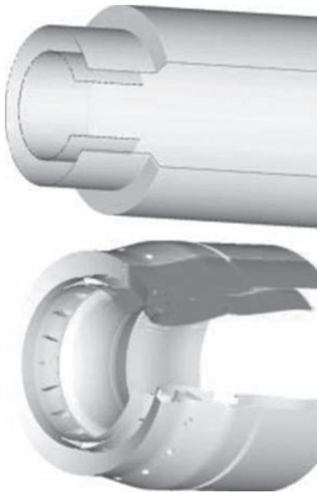
FIGURE 6.1 Schematics of an idealized coaxial dump combustor (top) and the combustor from a Pratt and Whitney gas-turbine engine (bottom). (Mahesh et al. 2006; with permission from ASME.)
