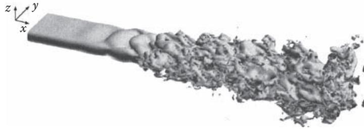
FIGURE 5.6 Snapshot of density isosurface: DNS of a transitional rectangular jet. (Rembold et al. 2002; with permission from Elsevier Science Ltd.)
