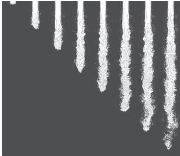
FIGURE 8.1 Turbulent atomization of a liquid diesel jet with  $\Delta t = 2.5''$  between each image. (Desjardins et al. 2008; with permission from Elsevier Science Ltd.)
